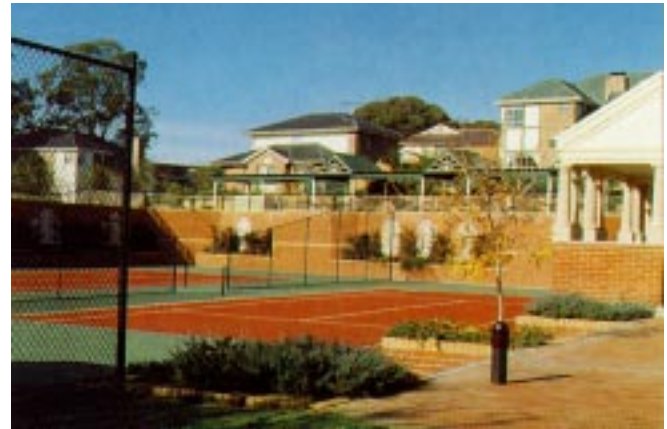
Figure 1: Tennis courts in this housing project in Sydney serve as a detention basin.
